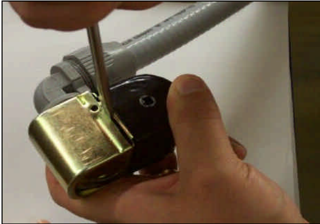
Prying open the coil wire cover
